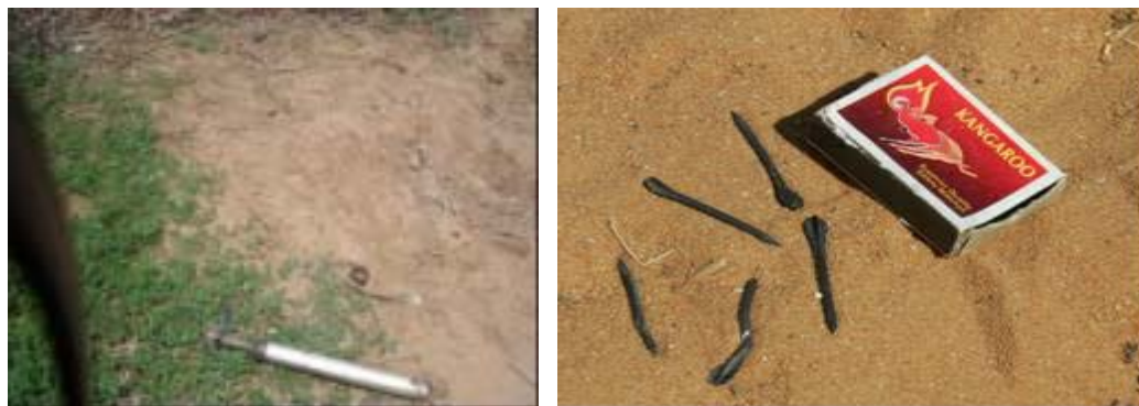
Figure 8 57-mm SKOG air-to-ground rocket (left) found at Abu Hamra and flechettes from SKOG air-to-ground rocket (right)
