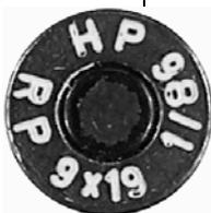
Marks on this cartridge identify the manufacturer (HP – Austrian manufacturer Hirtenberger Pat) and year of manufacture (/86 - 1986). Marks also identify the cartridge's unique lot number (1), its calibre (9mm x 19) – a widely used calibre for handguns – and a code allowing the manufacturer to identify the original recipient (RP - a German police unit).
